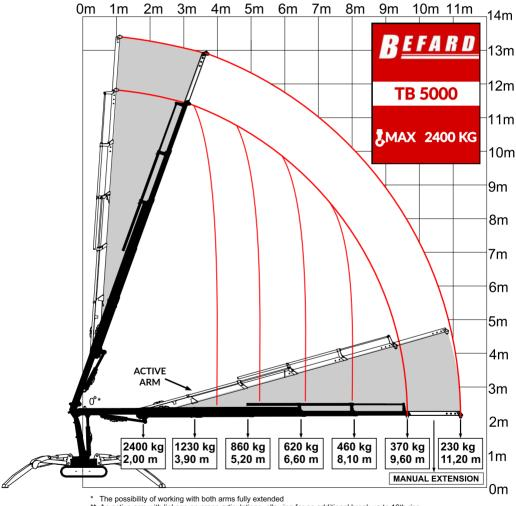
\*\* An active arm with linkage on crane articulations, allowing for an additional break up to 16th rise
