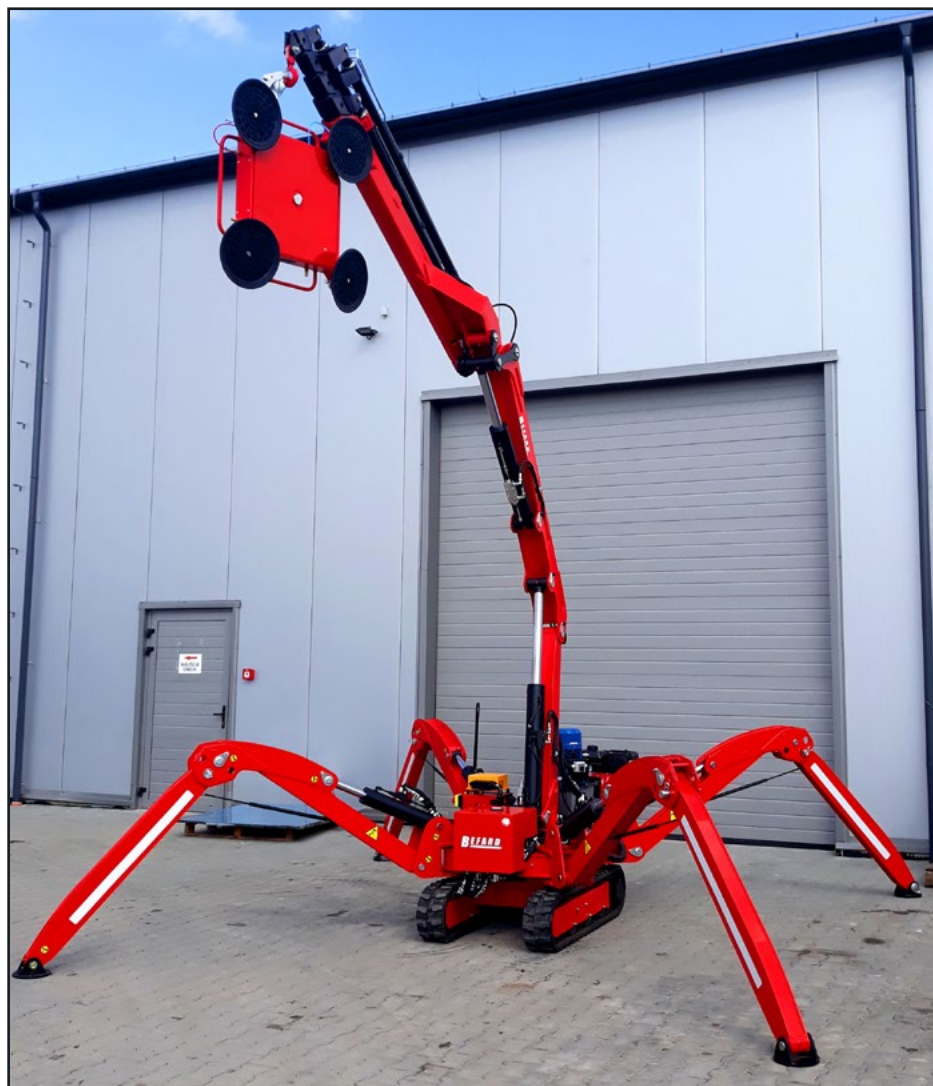
BEFARD TB MINI-CRANE ON CATERPILLAR CHASSIS
