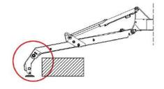
possibility of extending the supports to bypass the obstacle
